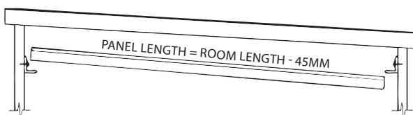
**Panel Width :** To balance the ceiling look and to avoid fitting a narrow strip at one end, check measure the room length and if necessary adjust/cut the first and last panel widths making sure you keep the male joint on the first panel and the female joint on the last panel.
